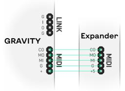
For the legacy connector, use 4 DuPont jumpers to connect matching pins as shown. Since it lacks a +5 pin, connect the power ribbon to the bus with a +5V line, aligning the ribbon's red line with the marking by the power connector.
